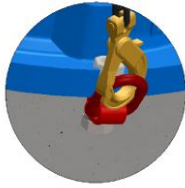
Figure 4-3 – Additional eyebolts detail for rib-cooled motor handling (not supplied with the motor)
