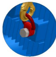
Figure 4-3 – Additional eyebolts detail for rib-cooled motor handling (not supplied with the motor)
