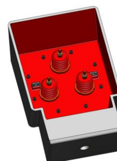
Figure 8-14 – Inside view of PTB
