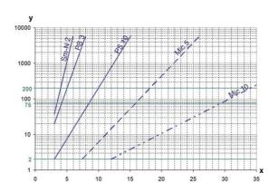
y = beta-value x = particle size [µm] determined by multipass tests (ISO 16889) calibration according to ISO 11171 (NIST)
