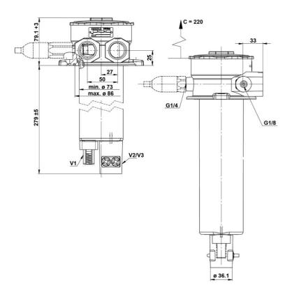
C = dismantling height required 220 mm
