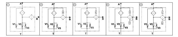
V1 = bypass valve V2 = preloaded valve
