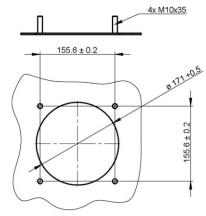
Fig. Tank cover connection
