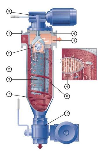
The filter is cleaned either when a preset differential pressure limit is reached or after a specified cycle time elapses. The FGC cartridge is rotated against a spring actuated scraper for this purpose. The special cartridge gap geometry guarantees efficient cleaning.
