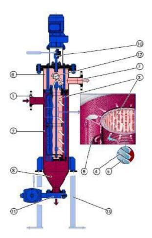
The filtered fluid exits the filter housing at the top opposite the inlet connection. In the AF 93 S version, the integrated preseparator relieves the filter cartridge of coarse and heavy particles by means of a tangential flow around the tube.
