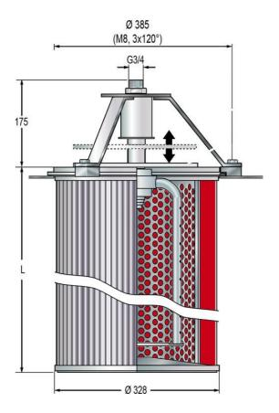
Installation on the cleaned gas side A hole with a diameter of 330 mm must be drilled in the filter plate.
