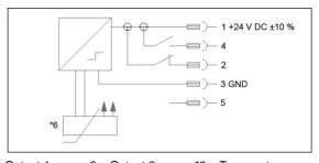
4 = Output 1 2 = Output 2 \*6 = Temperature sensor
