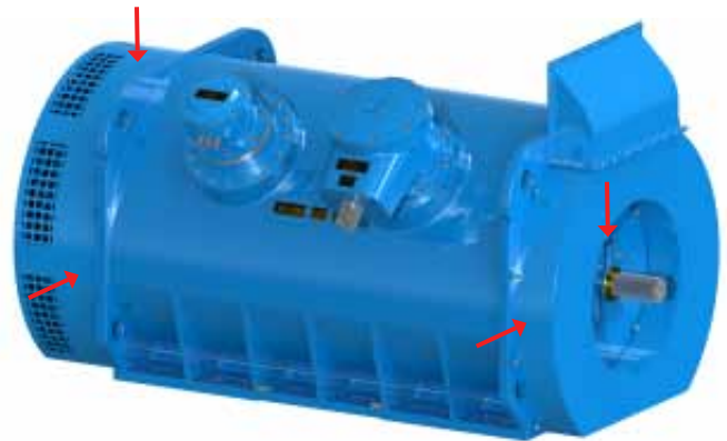
Figure 3.15 - Vibration monitoring directions on W22Xd tube-cooled motor
