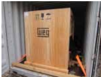
Figure 8.04 – Stuffing with lashing direct to motor eyebolts
