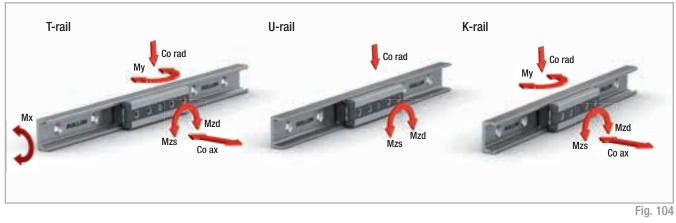
The load capacities in the following tables each apply for one slider. When using the slider in U-rails (floating bearing rails) the values are  $C_{_{0ax}}=0,\,M_{_x}=0$  and  $M_{_y}=0.$  When using the sliders in K-rails (compensation rails) the value is:  $M_{_x}=0.$
