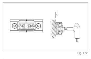
(5) The bottom of the rails should be supported in the area of the transition. Here a possible existing gap must be looked for, which must be closed for correct support of the rail ends by shims.
