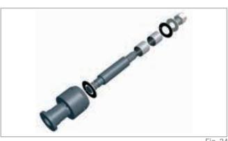
Important: remove the spacer washers to enable self-alignment of the roller slide
