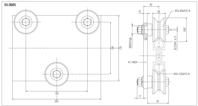
The plates - cod. 411.0825 and 411.0824 - are made in aluminium alloy with hard anodization. The rollers cod. 55.0760 4 rollers ROL-C062VC-BH + ROL-E062VC-BR and 55.0759 3 rollers ROL-C062VC-BH + ROL-E062VC-BR and/or different combinations from the ones shown on this page can be mounted on the above plates. Please call our technical dept. Prior any configuration changes.
