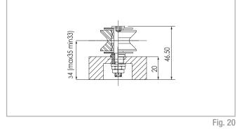
55.1066 - Roller assembly with one conc. axial free roller 55.1065 - Roller assembly with one ecc. axial free roller Max. Load per roller: radial 270 N No axial loading
