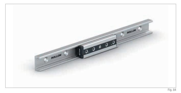
Compact Rail is the product family of guide rails consisting of roller sliders with radial bearings which slide on the internal, induction hardened and ground raceways of a C-profile made from cold-drawn roller bearing carbon steel.
