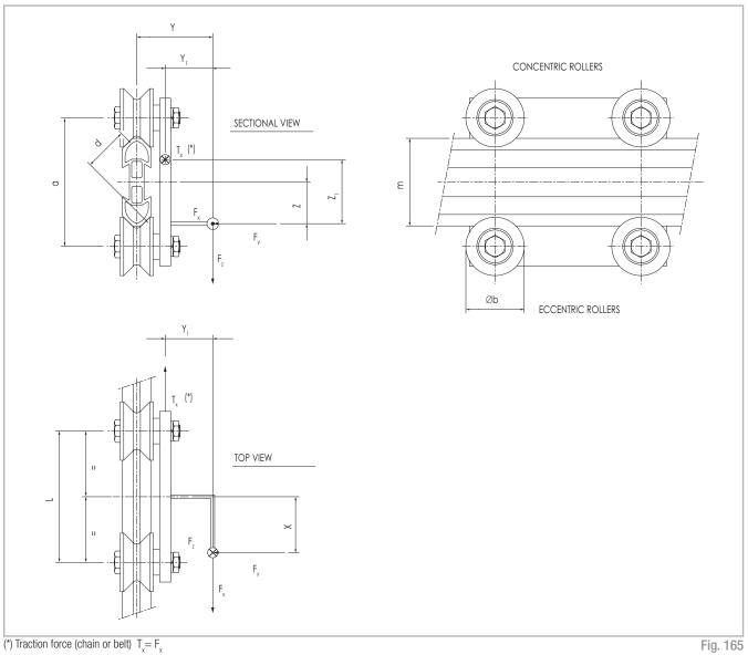
The rollers with concentric sleeve are mounted where there is the highest load and the ones with eccentric sleeve on the opposite end.
