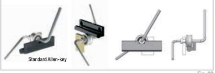
In case required to have eccentric rollers on the internal rail side, it is necessary to include optional accesses, code FXRG-....C, to allow Allen-key to reach the roller. Otherwise the adjustment can take place outside of the rail.
