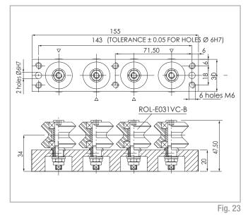
55.1069 - Roller assembly with 4 rollers, 2 conc. and 2 ecc. Max. load per roller: radial 270 N / axial 100 N
