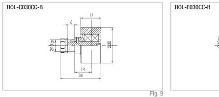
Plastic compound eccentric contrast roller, max radial load 200 N
