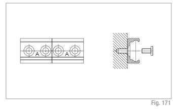
(3) Place the alignment fixture on the rail joint and tighten both set screws uniformly, until the raceways are aligned (see fig. 172).
