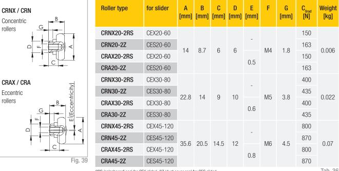
2RS (splashproof seal for CEX slider), 2Z (dust cover seal for CES slider)
