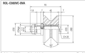
Radial load: 1000 N max. - lifetime lubrication
