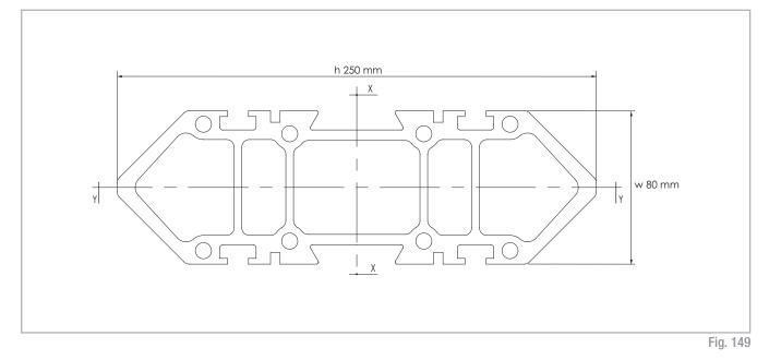
Surface quadratic moment X-X axis = 27.345.460 mm4 / Y-Y axis = 4.120.150 mm4.
