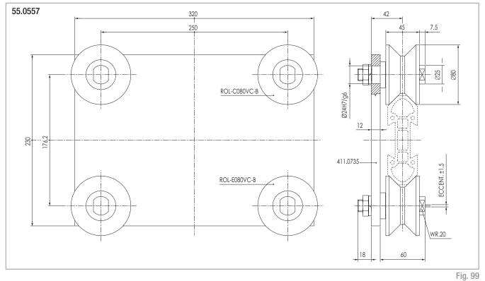
Roller assembly with 4 high stiffness rollers
