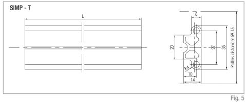
Drilled Speedy Rail 35 guide - Order code 411.1405/length in mm.
