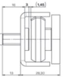
Limit towards inside of rail with TORX DIN 7991 screws
