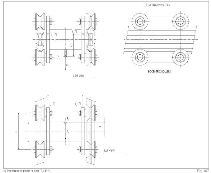
When assembling lines with parallel rail and long strokes it would be wise to use axially-free roller assemblies on one of the rails in order to withstand minor misalignments due either to assembly or maintenance errors. All 'F' values must include the dynamic component obtained by: Inertia Force = mass (kg) x acceleration (mt/s<sup>2</sup>).
