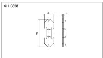
**Note:** drillings on the guide end are required as a safety measure with end-to-end joining in moving rails.
