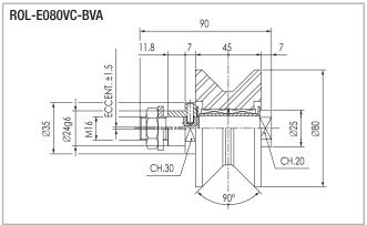
Radial load: 1000 N max. - lifetime lubrication
