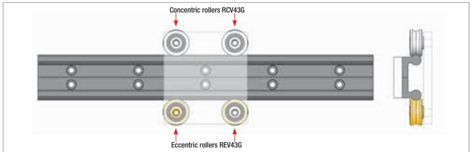
The rollers need to be positioned on the rail in numbers and directions according to the prevailing load. It is always preferable to orient the rollers so that the prevailing load acts radially, due to higher radial load capacity.
