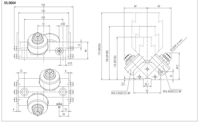
Light alloy compact roller assembly periodical lubrication version
