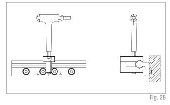
(5) The bottom of the rails should be supported in the area of the transition. Here a possible existing gap must be looked for, which must be closed if necessary for correct support of the rail ends by shims.
