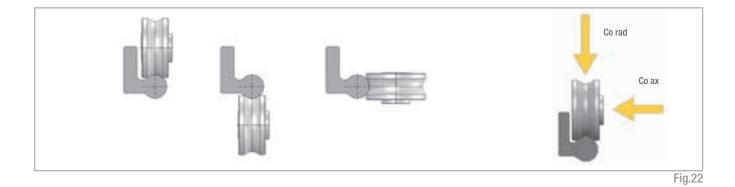
The rollers must be fixed on a metal surface not yielding, perfectly flat and with its fixing screws, applying a locking torque of 22 Nm.
