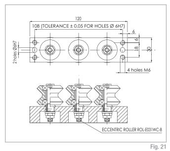
55.1060 - Roller assembly with two concentric rollers and one eccentric roller Max. load per roller: radial 270 N / axial 100 N
