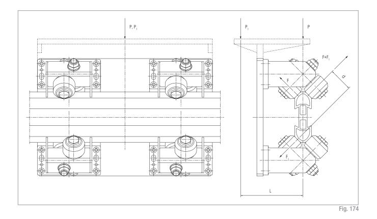
Rollers load with 'P' force applied on the rail axle
