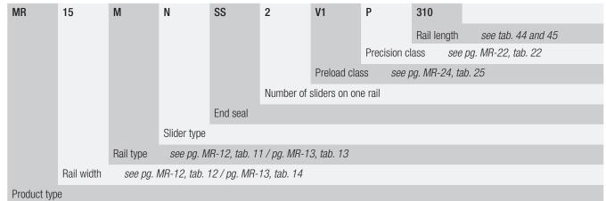
Ordering example: MR15MN-SS-2-V1-P-310 Hole pattern: 15-7x40-15, see fig. 61, tab. 44 / fig. 62, tab. 45
