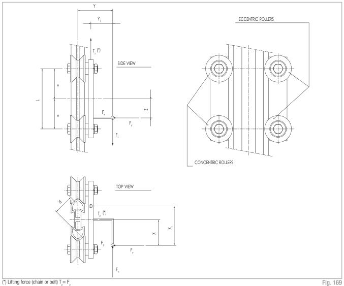
The rollers with concentric sleeve are mounted where there is the highest load and the ones with eccentric sleeve on the opposite end.
