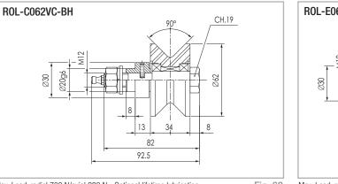
Max. Load: radial 700 N/axial 280 N - Optional lifetime lubrication
