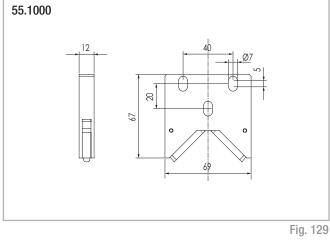
Scraper for blindo beam roller assemblies
