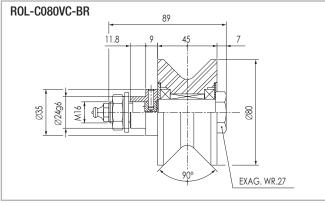
Radial load 1000 N max. axial load 400 N max. - Optional lifetime lubrication \$Fig. 89\$ (end play 0.010/0.030 mm)\$
