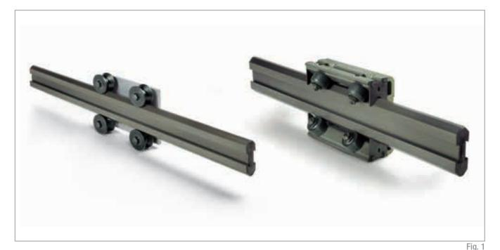
**Speedy Rail**<sup>®</sup> beam is a heat-treated aluminium alloy profile with hollow cross-sections which makes it very strong under torsion and deflection stresses. Beams are then subject to a special patented treatment which provides a smooth, hard (700 HV) surface comparable to tempered steel. The fusion point of the non-stick surface layer (2100°C) permits an excellent resistance to welding splatters.
