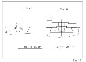
Roller assembly with "V" shaped rollers
