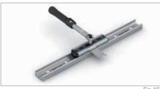
(6) By turning the flat key clockwise, the roller to be adjusted is pressed against the upper track and the slider is then without play. Avoid a preload that is too high. It generates increased wear and reduces the service life.
