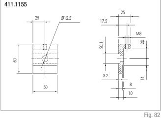
For rack mounting plate mod.3 Use dovetaile 411.1111
