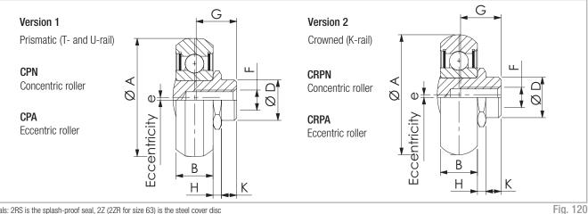
Seals: 2RS is the splash-proof seal, 2Z (2ZR for size 63) is the steel cover disc Note: The rollers are lubricated for life
