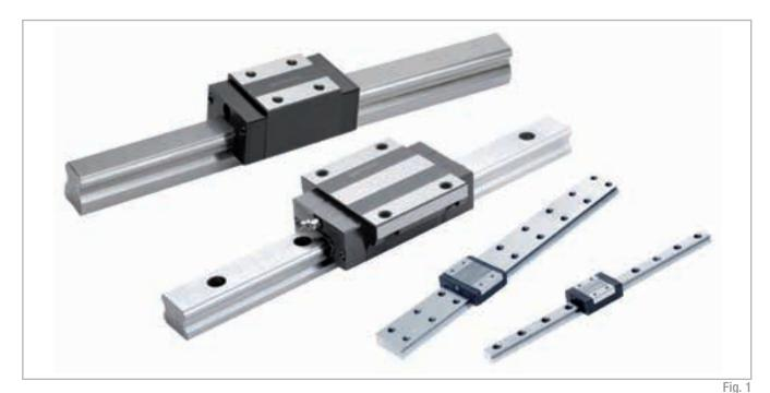
The running grooves are ground in semicircular profile and have a contact angle of 45° in X-arrangement so that the same load capacity is guaranteed in all principle directions. Use of large steel balls enables high load and moment capacities. All carriages in size 55 are equipped with ball chains.
