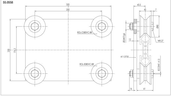
The plate -cod. 411.0735 - is made in aluminium alloy with hard anodization. The rollers -cod. ROL-C080VC-BVA ROL-E080VC-BVA, carriage cod. 55.0636, - and/or different combinations from the ones shown on this page can be mounted on the above plates after consulting our technical department.
