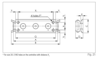
Y<sub>1</sub> [mm] **X**<sub>2</sub> [mm] Υ<sub>2</sub> [mm] Α В С D Е F G Weight X<sub>1</sub> **Slider type** Size [mm] [mm] [mm] [mm] [mm] [mm] [mm] [kg] CES20-80 20 80 90 71 60 9 0.05 18 11.5 5.5 M5 5.5 -CES30-88 30 88 97 27 15 4.5 M5 80 70 5 15 6 0.11 CES45-150 45 150 160 40 22 4 M6 135 120 7.5 23 8.5 0.40
