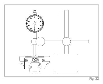
Preload is defined as an effective load on the rolling element in the interior of the carriage in order to remove an existing clearance or to increase the rigidity.
