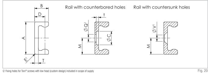
Q' Fixing holes for Torx® screws with low head (custom design) included in scope of supply V' Fixing holes for countersunk head screws according to DIN 7991
