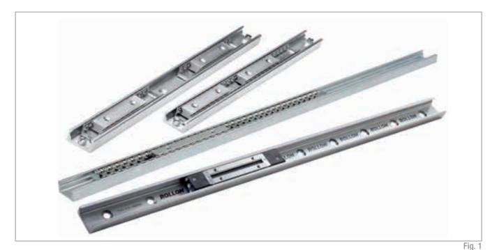
The Easyslide series is a system of drawn steel linear rails with induction hardened raceways. The system consists of an "C" shaped linear profile rail, and one or more internal sliders with caged recirculating ball bearings.
