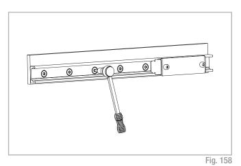
(2) Install a dial indicator so that the offset of the rail to a reference line can be measured. Now position the slider in the center of the rail and set the dial indicator to zero. Move the slider back and forth between each two hole spacings and carefully align the rail. Fasten the three center screws of this area now with the the specified tightening torque, see pg. fig. 159.(3) Now position the slider on one end of the rail and carefully align the rail to zero on the dial indicator.
