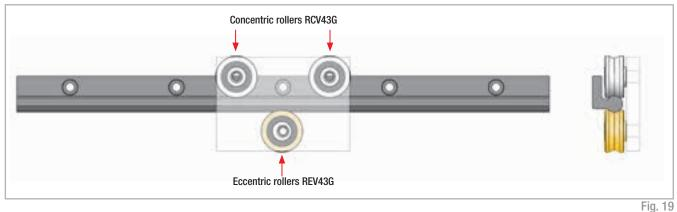
It is recommended, when more than two rollers are on the same track with max. radial load, to use only two concentric rollers (as from example figure). The others should be eccentric. For cases with a wider distance between concentric rollers, please contact ROLLON's Technical departement for dimensioning.
