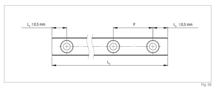
Hole pitch P [mm] L<sub>2max</sub>\*, L<sub>3max</sub>\* [mm] Size L<sub>2min</sub>, L<sub>3min</sub> [mm] L<sub>omax</sub> [mm] 15 7 20 4000 60 25 20 30 80 8.5 3960 35 45 11.5 22.5 3930 105 55 120 13 30 3900
