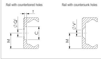
Q1 Fixing holes for Torx<sup>®</sup> screws with low head (custom design) included in scope of supply
