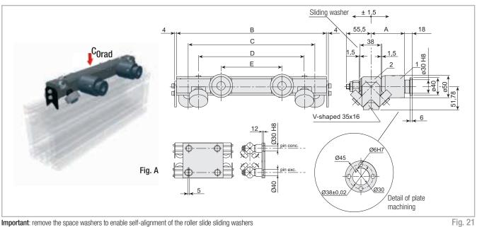
Important: remove the space washers to enable self-alignment of the roller slide sliding washers
