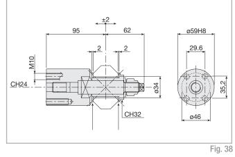
Important: remove the spacer washers to enable self-alignment of the roller slide
