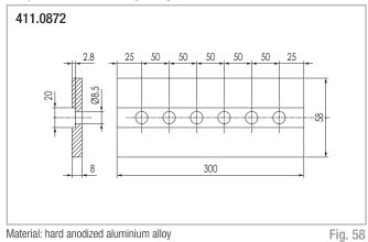
Steel plate for m2 rack mounting
