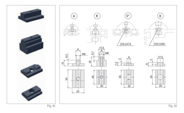
\* Special drilling for M8 screws instead of M10 is required.
