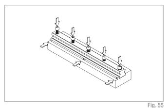
(3) Tighten the thrust bolts on the guide rail until there is close contact on the side stop surface (see fig. 56).
