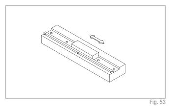
(2) Carefully lay the guide rail on the assembly surface (see fig. 54) and slightly tighten the fixing screws so that the guide rail lightly touches the assembly surface (align the guide rail along the shoulder edge of the assembly surface, see fig. 55).
