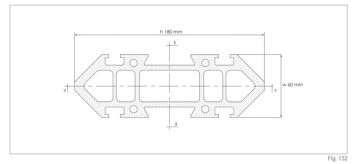
Surface quadratic moment: X-X axis = 10.291.100 mm4 / Y-Y axis = 1.278.700 mm4.
