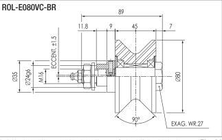
Radial load 1000 N max. axial load 400 N max. - Optional lifetime lubrication  $$Fig. \,90$$  (end play 0.010/0.030 mm)
