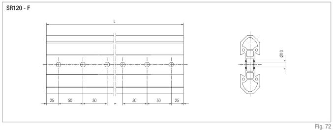
**Note:** drillings on guide end are required as a safety measure with end-to-end joining in moving rails.
