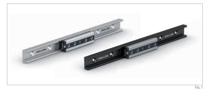
Featuring double row ball bearings, new rigid rails with convex raceways and new robust steel sliders with longitudinal protection and floating wipers, Compact Rail Plus has been designed for the most demanding applications in terms of load capacities, dynamics and work environment. All while maintaining the self-aligning capabilities that make this product family unique.
