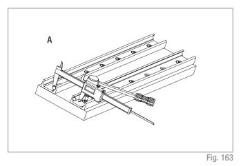
(3) Fasten the rail in Position B so that the distance between the raceways does not exceed the measured values in Position A while maintaining the tolerances (see pg. CR-93, tab. 78) for parallel rail installation.
