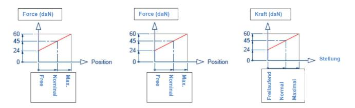
The suspended fork produces a force on the wheel, maintaining it in contact with the floor.
