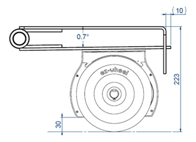
Diagram showing the mounting height under the application chassis in the nominal position
