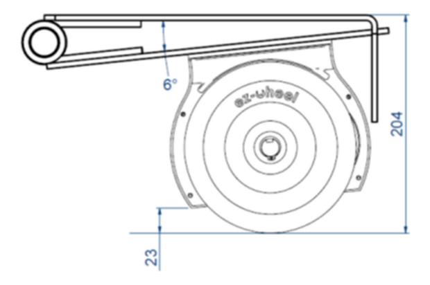
If skidding is observed despite the force applied by the suspended fork, check that the rest position of the suspended fork is the nominal position.
