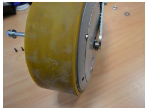
• Fix the M16 screw with the M16 nut supplied.
