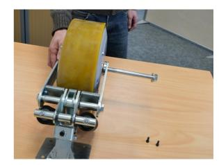
■ Insert the holding ring between the fork and the wheel on the opposite side from the anti-rotation washer.
