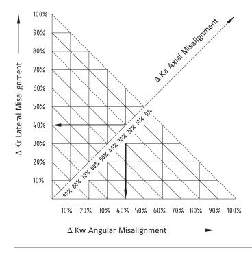
Prior to installation, the shaft misalignment must be measured. Each type of misalignment (axial / lateral / angular) must be calculated and checked against this chart.
