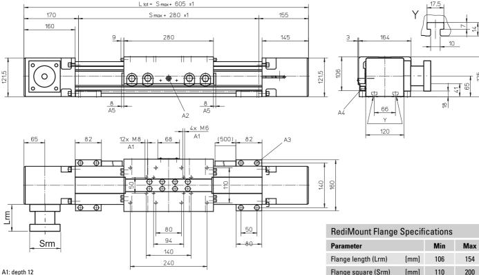
A2: funnel type lubricating nipple DIN3405-M6×1-D1
